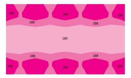
Average: 187 μMol/m<sup>2</sup>/s Maximum:194 μMol/m<sup>2</sup>/s Minimum:180 μMol/m<sup>2</sup>/s Uniformity: 92%
